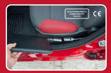
The tip-up plate is easily removable. A security system automatically stops the tip-up plate stroke in case of need. Maximum load is 100 Kiloes.
